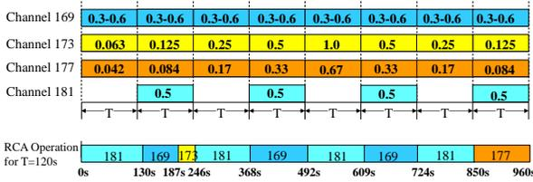
Fig. 7: Traffic pattern generated for RCA evaluation
