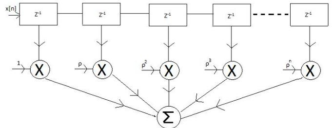
Fig. 1. Tapped delay line model for wideband wireless systems
