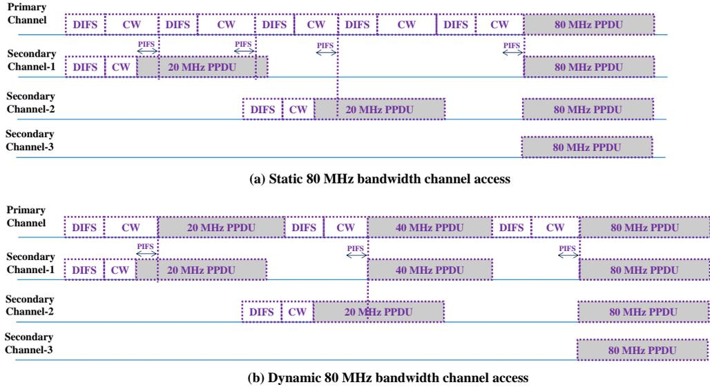
Fig. 4: Channel access mechanism for primary and secondary channels in 802.11ac
