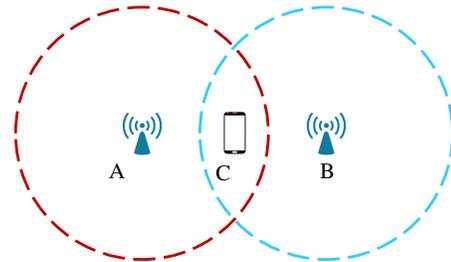
Fig. 7: A diagram illustrating the hidden node problem. Stations A and B are trying to communicate with Station C. However, Stations A and B cannot “hear” each other as they are out of each other’s sensing range. In such cases, it is possible that Station C receives signals from A and B simultaneously resulting in packet collisions.
