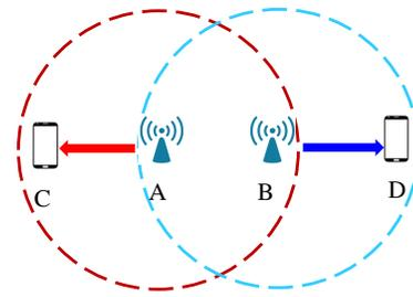
Fig. 10: A diagram illustrating the exposed node problem. Stations C and D are outside each others’ sensing and transmission range. Thus, A and B can transmit packets to C and D respectively without any collisions. However, B (or A) senses A’s (or B’s) transmission to C (or D) and does not transmit, resulting in loss of an opportunity to transmit.
