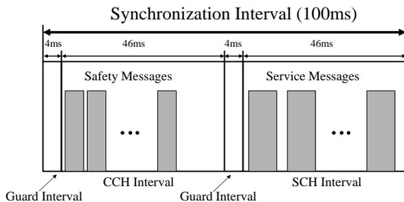
Fig. 6: The multichannel MAC scheme used by DSRC
