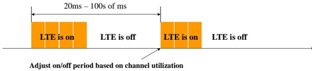
Fig. 9: CSAT process
