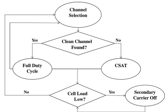
Fig. 8: LTE-U algorithm flow chart
