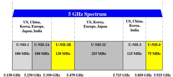
Fig. 1: Unlicensed spectrum and regulations in the 5 GHz band. Regions marked yellow are U-NII bands proposed to open up for use by unlicensed devices in US. NPRM 13-22.
