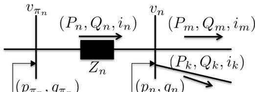
Fig. 1: Node in radial distribution grid
