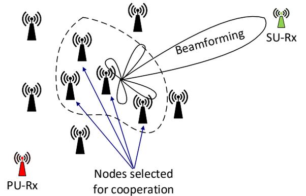
Figure 2. Desired beampattern with node selection.
