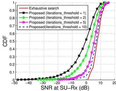
Figure 7. Performance comparison: proposed scheme vs. exhaustive search
