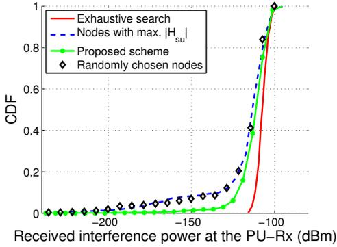
Figure 6. CDF of interference power at the PU-Rx ( $N_T = 15, N = 5$ )
